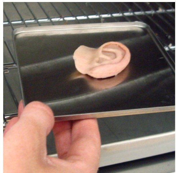
Step 4 - oven cure inks at 110°C for 15 minutes
