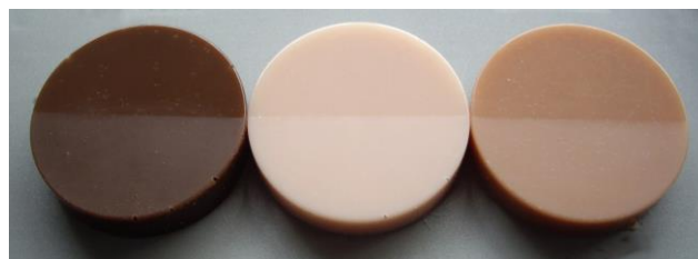
Fig 12: Shows three typical skin tones in cured silicone. The top half is smooth and glossy, the bottom half has a rougher matt finish. The affect that surface texture has on the direction of light and in turn the colour is clear to see.
